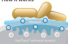
Silver ions embedded in the material substrate are released via ambient moisture and enter the cell membrane. The silver ions destabilise the cell, stop respiration and inhibit cell division, whilst blocking the replication of DNA, killing the cell.
