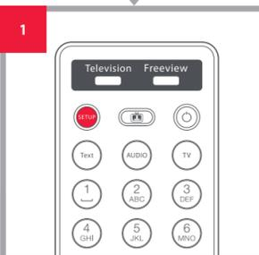
Press and release the TV key. Then hold down the SETUP key until the TV key blinks twice.
