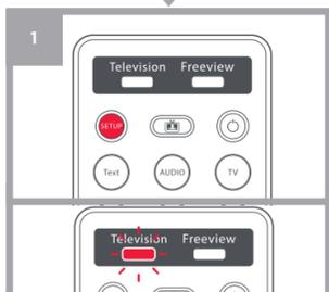
Press and release the TV key. Hold down the SETUP key until the TV key blinks twice.
