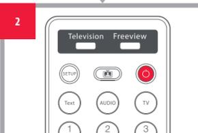
Point the remote at your TV. Press and hold the POWER key. The remote will send a different Power signal to your TV every 3 seconds. As soon as the TV switches off, release the Power key to store the code. The LED will blink twice, and the remote should now operate your TV. If you find that some keys operate incorrectly or not at all, repeat from Step 1 to find the next code.
