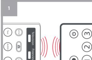
Place the original remote facing the One For All remote on a flat surface.
