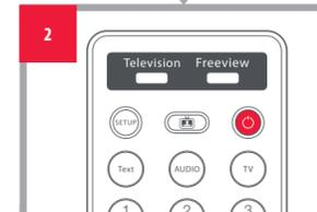
Point the remote at your Freeview/ Freesat box. Press and hold the Power key. The remote will send a different Power signal to your box every 3 seconds. As soon as the Set Top Box switches off, release the Power key to store the code. The LED will blink twice, and the remote should now operate your box. If you find that some keys operate incorrectly or not at all, repeat from Step 1 to find the next code.
